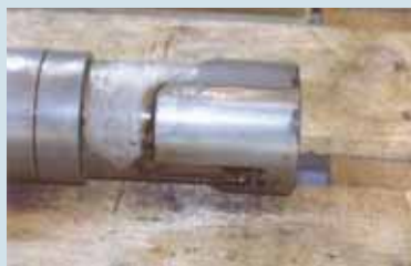
Fuel pump plunger sticking by use of Low Sulphur Fuel. (Source MAN Diesel "Operation on Low-Sulphur Fuels Two-Stroke Engines")
