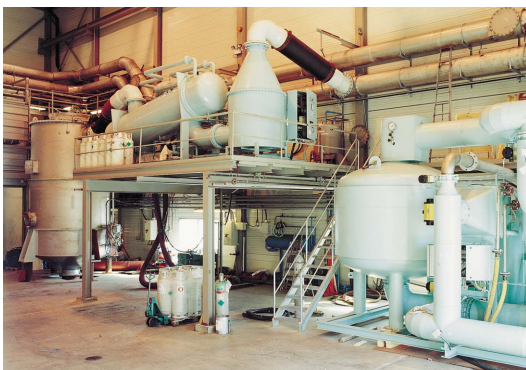
Testing of an inert gas generator with cooling drier and absorption drier for an LNG carrier. 14,000 Nm 3 /h inert gas with dew point -45°C
