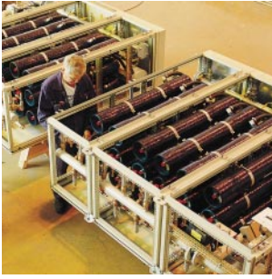
Assembly of membrane cabinets
