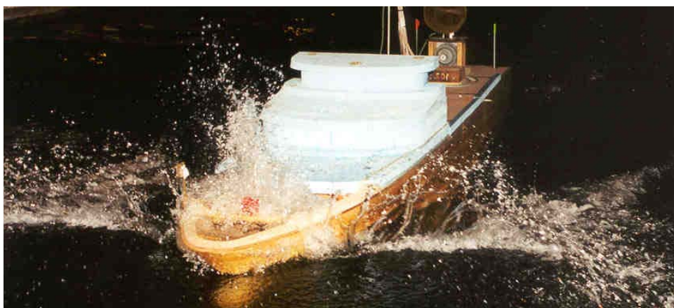
Seakeeping tests for a large luxury yacht in DMI's large towing tank
