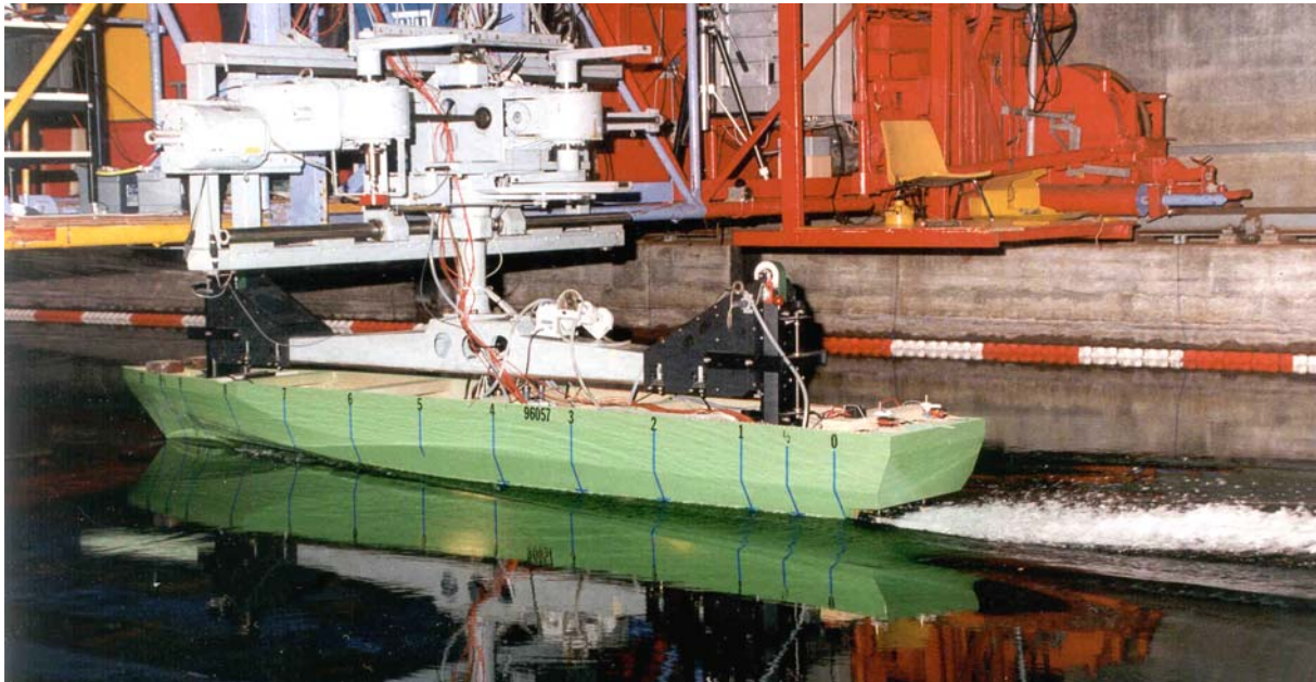
Manoeuvring tests in PMM setup with waterjet powered vessel
