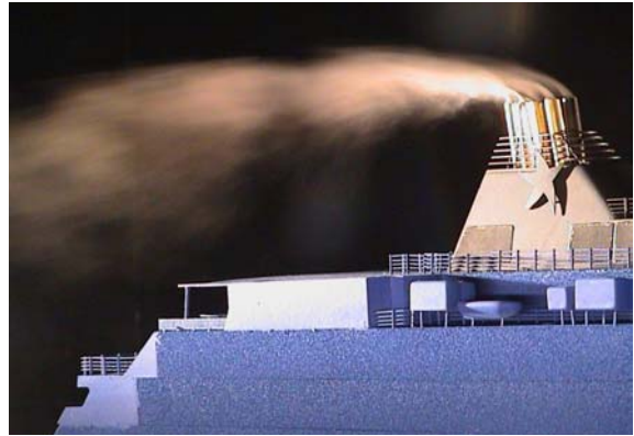
Smoke tests for funnel design
