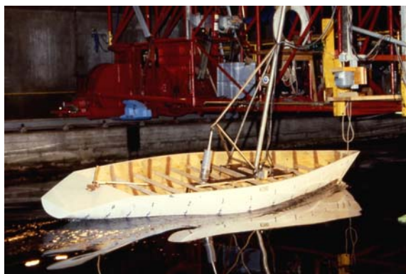
Sailing yacht in the towing tank
