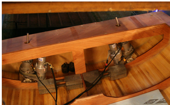
Steering system installed in a twin rudder yacht
